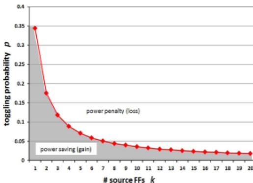
Fig.7. Power saving breakeven curve
