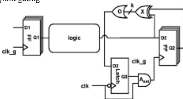
Fig.1. Circuit implementation of data – driven clock gating
