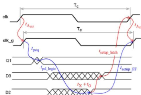
Fig.2. Sequencing of gating logic in data driven Clock gating
