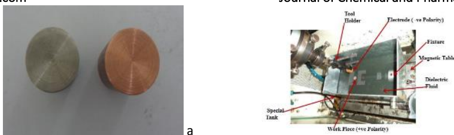
Figure.1a & 1b. shows copper and silver coated tool, Experimental Setup.
