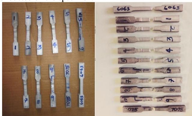
Figure.5. Tensile Test specimens before and after testing
