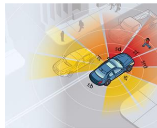
Figure.2. Proposed system with sensors in all sides
