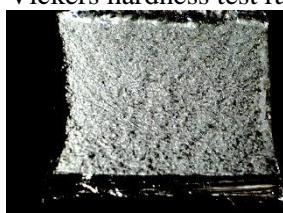
**Figure.7a.Grain boundary after impact test**
