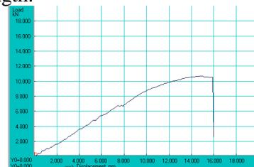
**Figure.6b. load-displacement (tensile)**
