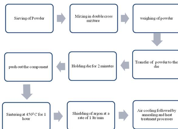
**Figure.3. Process flow sheet for Mg powder metallurgy**
