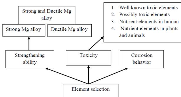
**Figure.2. Considerations for element selection in developing bio-Mg alloys**
