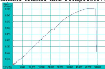
**Figure.6a. stress-strain (tensile)**
