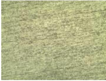
**Figure.3.**Micro examination of the parent region grains of ferrite with particles of alloy carbides present in the ferritic matrix
