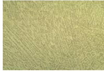
**Figure.4.**Micro examination of weld pool revealed dendritic delta ferrite
