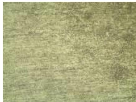
**Figure.2.**Micro examination of the parent region revealed grains of ferrite with particles of alloy carbides present in the ferritic matrix
