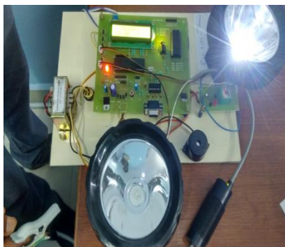
Figure.7.Heart beat Sensor measuring Heart Beat of a Patient and transmitting through Li-Fi
