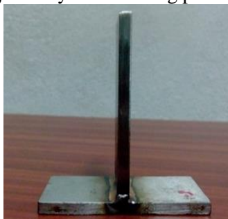
Figure.2. Welded T-joint material by TIG welding process
