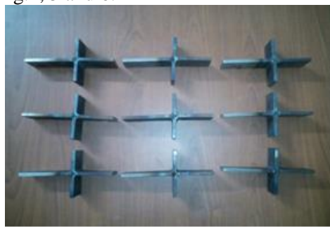
Figure.5. Nine types of t-joint weld section for testing purpose
