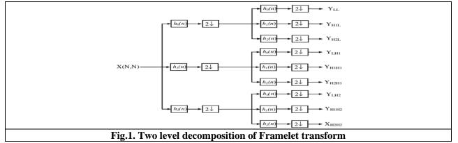
Framelets has higher incidence sieve banks to develop large sub bands in decomposition. Image fusion finds application in the field of navigation guidance, target detection, and recognition, medical diagnosis,
