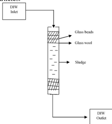
**Figure.1. Schematic representation of Column (not to scale)**
