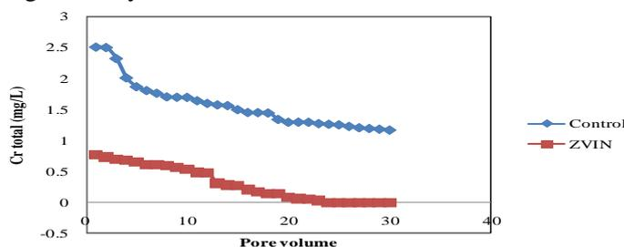
**Figure.3. Leachability of chromium from unamended sludge and sludge amended by ZVIN under dynamic condition**
