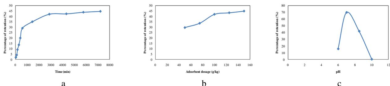
**Figure.2. Immobilization of chromium in tannery sludge with various parameters (a) Time (b) adsorbent dosage and (c) pH**
