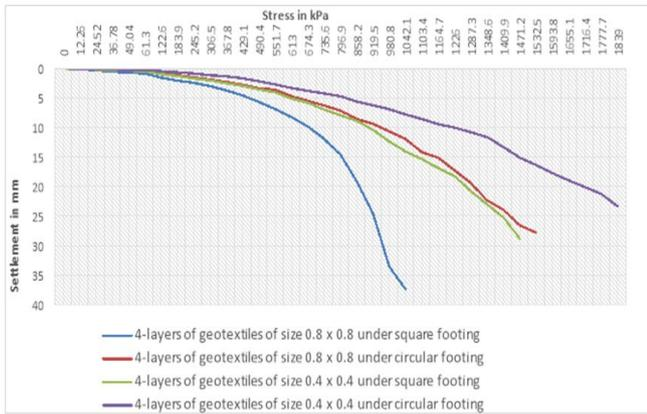
Figure.3. The relationship between stress and settlement of plate for determination of ultimate bearing capacity for square plate of 100mm x 100mm.
