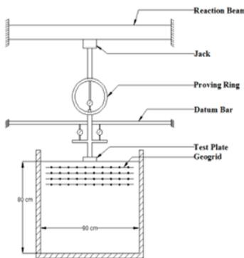
Figure.1. shows the test setup for granular soil as foundation bed
