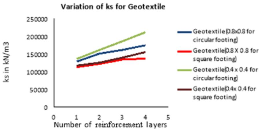
Figure.5. Values of  $k_s$  ( $\text{kN/m}^3$ ) of weak soil using Plate Load test under model circular footing(100 mm ) and model square footing (100mm x 100mm)
