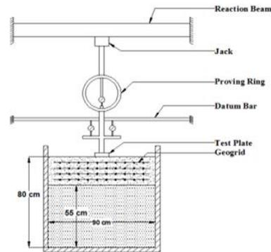
Figure.2. shows the test setup for weak soil as foundation bed
