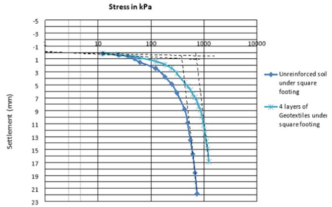
Figure.4. Values of  $k_s$  ( $\text{kN/m}^3$ ) of weak soil using Plate Load test under model circular footing(100 mm ) and model square footing (100mm x 100mm)
