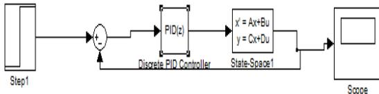
Figure.9. PID controlled system
