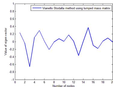
Figure.2. (b) showing the eigen frequency plot for each node at converged value.
