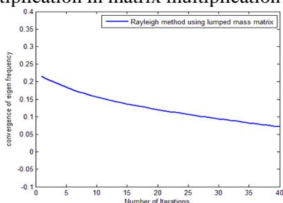
Figure.6. (a) Convergence of eigen frequency with nos. of iterative cycle
