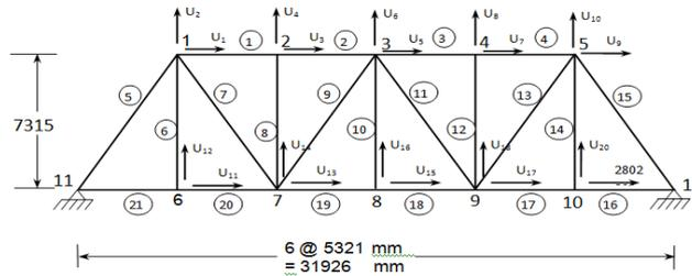
Figure.1. Railway bridge truss
