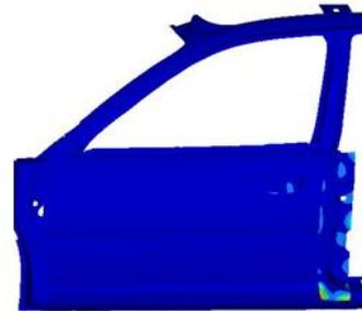
Figure.4. At mode -7 for free-free condition with stiffener
