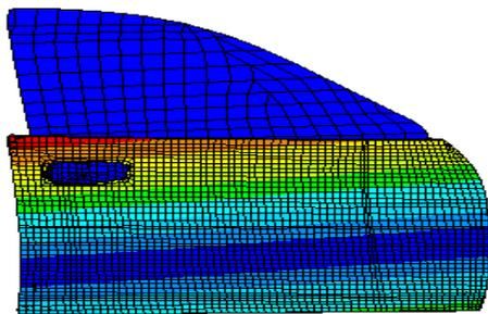
Figure.3. At mode-7 for free-free condition without stiffener
