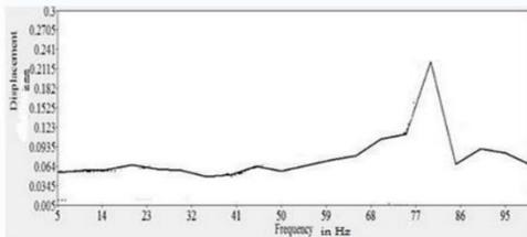
Figure.5. Harmonic analysis of door without stiffener
