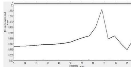
Figure.6. Harmonic analysis of car door with stiffener
