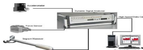
Figure.7. Experimental modal analysis measuring instruments
