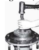
To instal inner oil seal in rear hub(8T & 10T)
