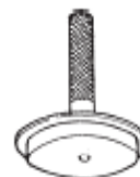
To instal inner oil seal in rear hub(8T & 10T)
