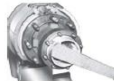
To tighten or loosen hub nut (8T & 10T)
