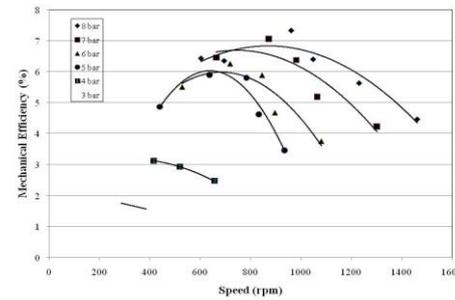
**Fig.7. Effect of Speed on Mechanical Efficiency for various Pressure**
