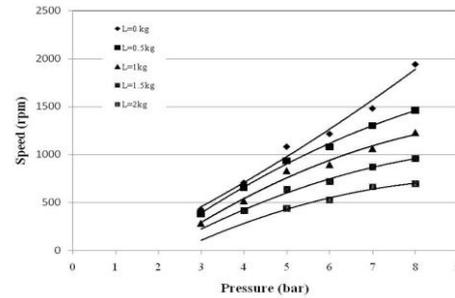
**Fig.5. Effect of Pressure on Speed for various loads**
