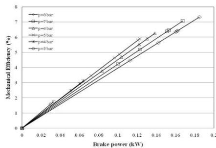
**Fig.6. Effect of Brake Power on Mechanical Efficiency for various loads**
