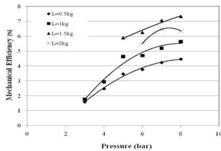
**Fig.4. Effect of Pressure on Mechanical efficiency for various loads**
