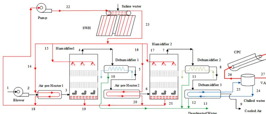
**Fig.1. Line diagram of two stage desalination plant**
