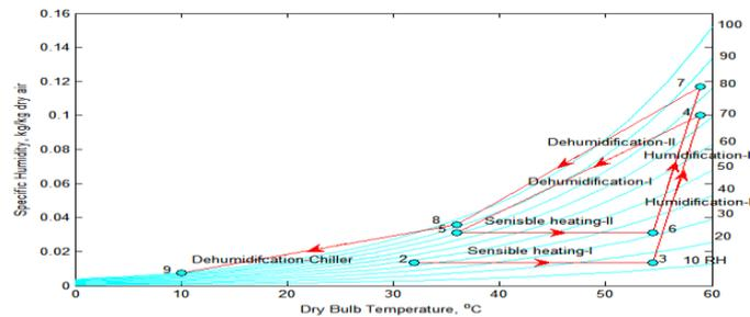
**Fig.2. Psychrometric processes in desalination plant**
