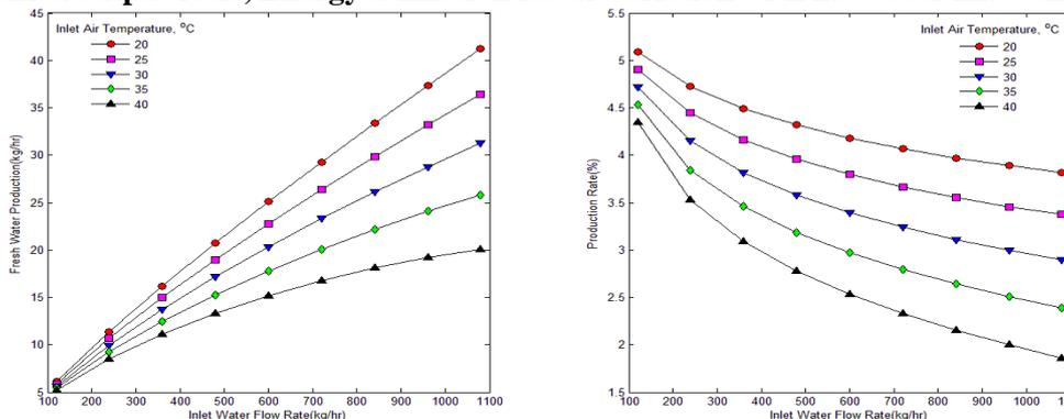
**Fig.4. Study on the influence of hot water flow rate on fresh water production and production rate**
