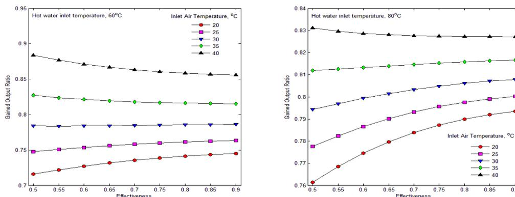
**Fig.5.Variation of GOR with humidifier effectiveness at air temperatures of 60°C and 80°C**
