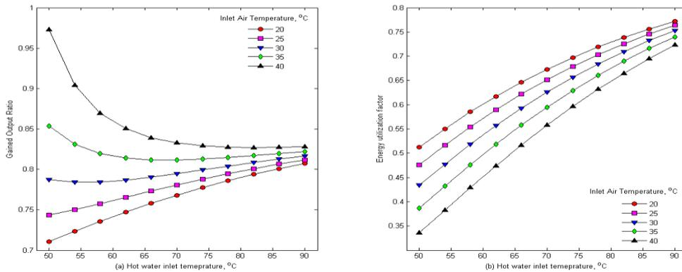
**Fig.3. Gained output ratio, Energy utilization factor variation with hot water inlet temperature**
