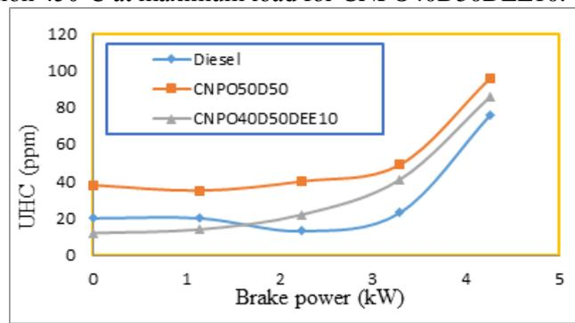
Fig.6. Brake power vs Hydrocarbon emission
