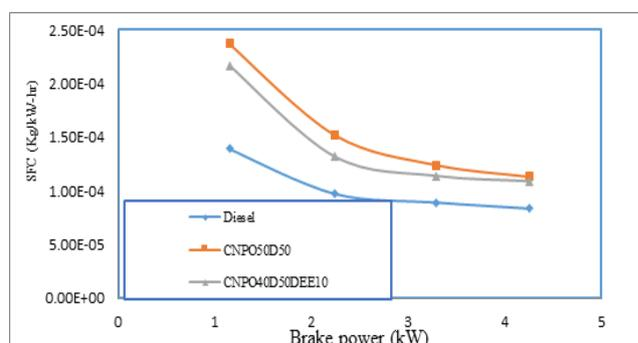
Fig.4. Brake power vs Specific fuel consumption
