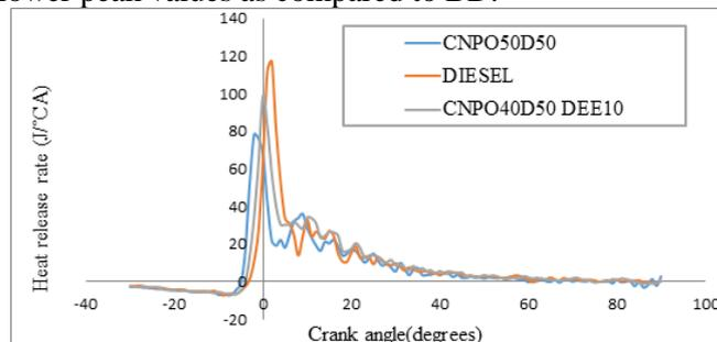
Fig.9. Variation of Heat Release Rate at Peak Power output
