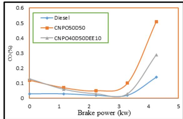
Fig.8. Brake power vs Carbon monoxide emission
