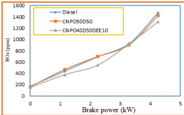
Fig.7. Brake power vs Nitrogen oxide emission
