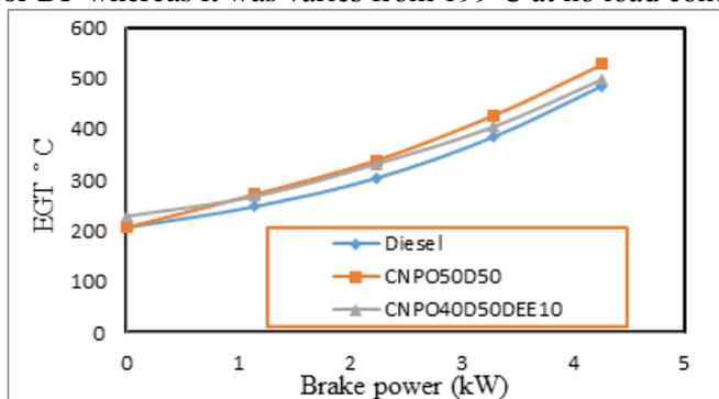
Fig.5. Brake power vs Exhaust gas temperature
