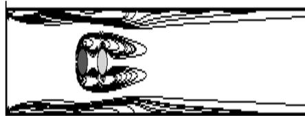
Fig.4. Vorticity contours of tandem arrangement at  $Re = 40$ .
