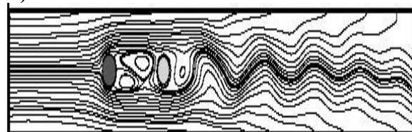
Fig.14. Instantaneous streamline patterns at  $Re = 100$ . (4.0D)
