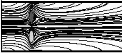
**Fig.19. Instantaneous streamline patterns at  $Re = 30$ .**
