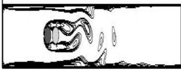
Fig.7. Vorticity contours of cylinders at  $Re = 100$  (1.5D)
