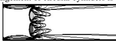
Fig.17. Vorticity contours of two circular cylinders at  $Re = 50$ .
