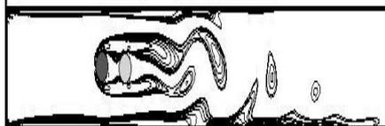
Fig.8. Vorticity contours of cylinders at  $Re = 100$  (2.0D)
