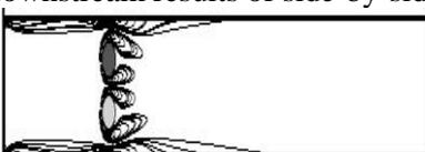
Fig.16. Vorticity contours of two circular cylinders at  $Re = 30$ .
