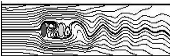
Fig.13. Instantaneous streamline patterns at  $Re = 100$ . (3.0D)
