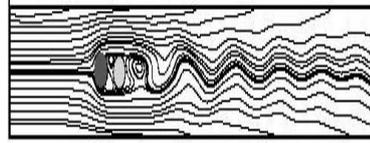
Fig.11. Instantaneous streamline patterns at  $Re = 100$ . (1.5D)
