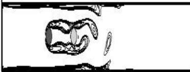
Fig.10. Vorticity contours of cylinders at  $Re = 100$  (4.0D)
