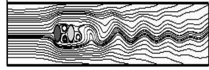
Fig.12. Instantaneous streamline patterns at  $Re = 100$ . (2.0D)
