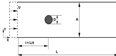
Fig.2. Schematic diagram of the flow past a circular cylinder.
