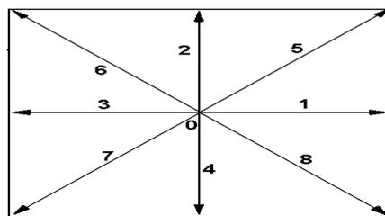
Fig.1. Two-Dimensional nine-velocity square lattice model.
