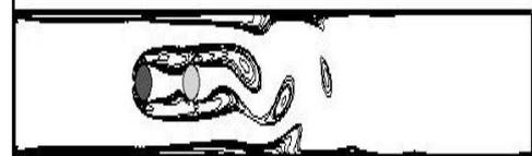
Fig.9. Vorticity contours of cylinders at  $Re = 100$  (3.0D)
