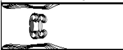
Fig.3. Vorticity contours of tandem arrangement at  $Re = 20$ .
