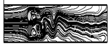
**Fig.21. Instantaneous streamline patterns at  $Re = 100$ .**
