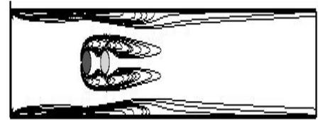
Fig.5. Vorticity contours of tandem arrangement at  $Re = 60$ .
