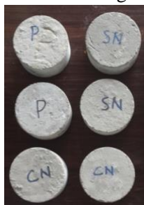
Figure.3. Typical M25 grade SCC concrete disc with different optimum % of corrosion inhibitors
