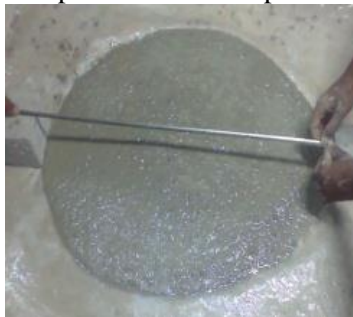
(a).Slump flow & T50 Test
