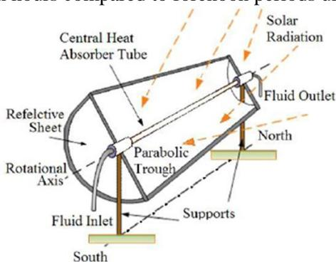
Fig.1. Schematic of single axis parabolic trough collector
