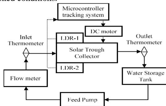
Fig.2. Schematic of the solar PTC experimental setup
