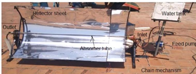
Fig.5. Solar Parabolic Trough Collector
