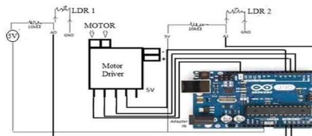
Fig.3. Microcontroller based solar tracking circuit for PTC
