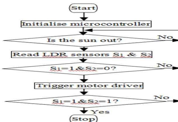
Fig.4. Solar tracking control algorithm
