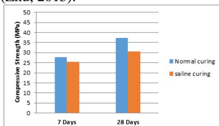
**Fig.3. Compressive strength for Mix 1**
