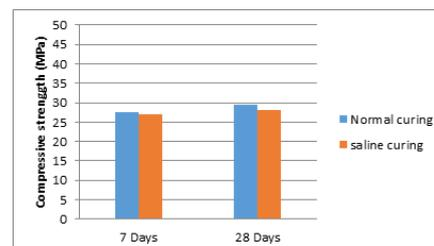
**Fig.4. Compressive strength for Mix 2**
