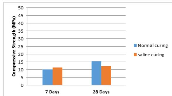
**Fig.7. Compressive strength for Mix 5**
