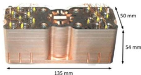
**Figure.2. Prototype of digital valves (Palonitty, 2014)**
