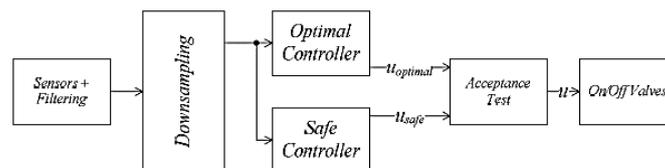
**Figure.5. Block diagram of the control strategy for fault tolerancing (Huova, 2010)**
