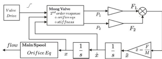
**Figure.3. Model of the digital valve spool (Linjama, 2009)**
