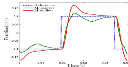
**Figure.4. Deviation between modelled and measured output of PID control (Linjama, 2009)**
