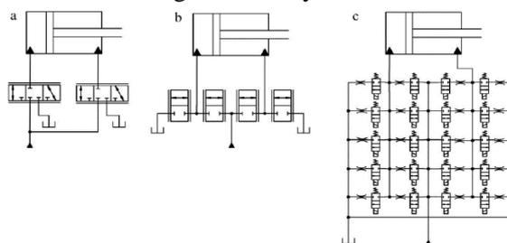
**Figure.1 a.2- three way proportional valve distributed system; (b) 4- two way valve system; (c) a digital on-off valve system (Linjama, 2012)**
