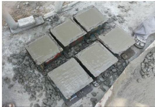
Fig.1. Shows the cubes after casting
