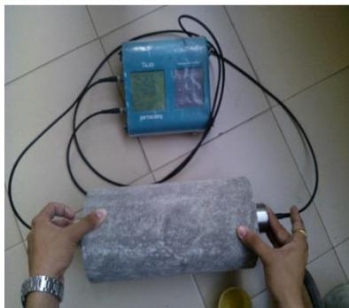
**Fig.2. Testing of specimen using NDT**
