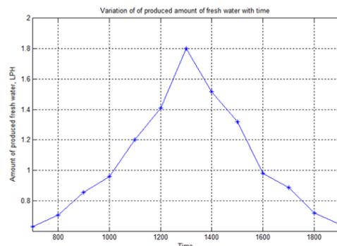
**Fig.8. Average amount of produced water from 2nd dehumidifier with different time of the day**
