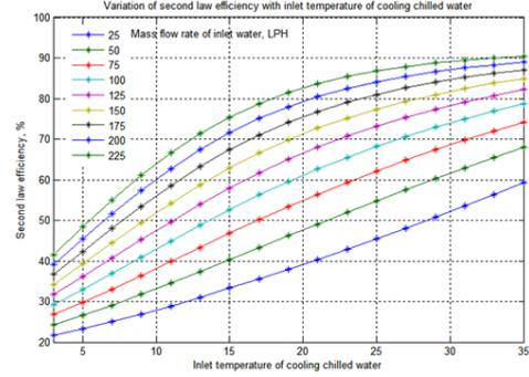
**Fig.6. Variation of exergy efficiency with inlet chilled water temperature.**
