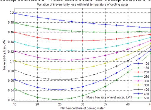
**Fig.3. Variation of Irreversibility loss with change in temperature of cooling water**
