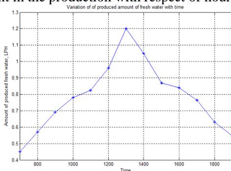
**Fig.7. Average amount of produced water from first dehumidifier with different time of the day**
