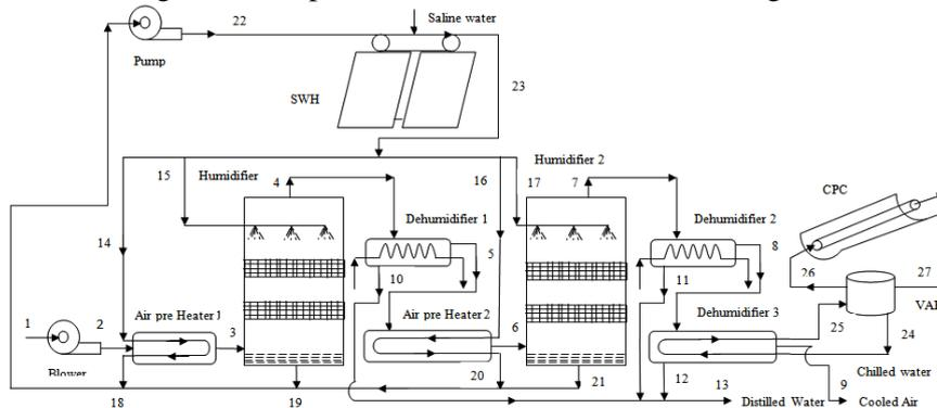
**Fig.1. Schematic diagram of two stage desalination plant**
