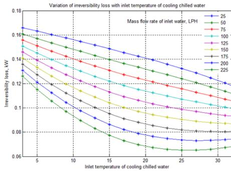
**Fig.5. Variation of irreversibility loss with inlet chilled water temperature**
