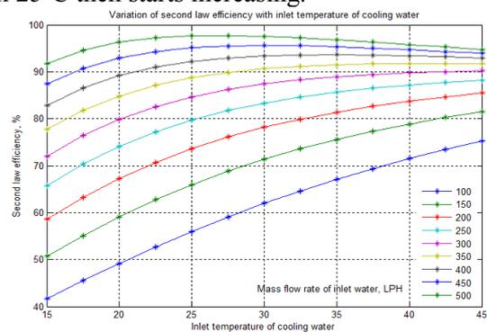
**Fig. 4. Variation of exergy efficiency with variation in temperature of cooling water**
