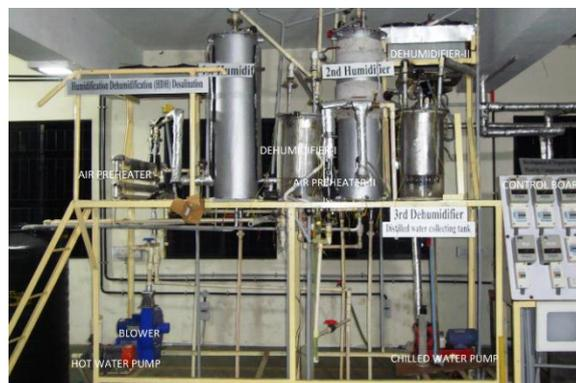
**Fig.2. Experimental setup with instrumentation**
