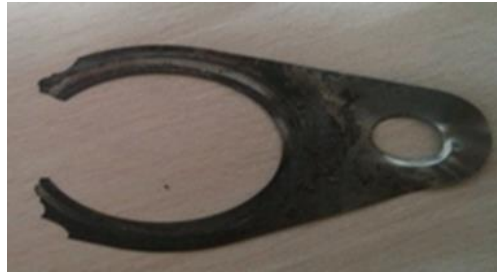
Fig.2. Evidence of no gap failure in an exhaust manifold gasket leading to wear at one end
