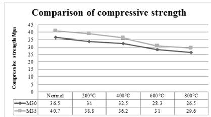
**Graph.1. Comparison of compressive strength at various temperature**
