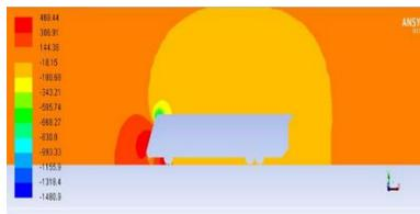
**Figure.7b. Static Pressure (Pa) Plot for Model-D**
