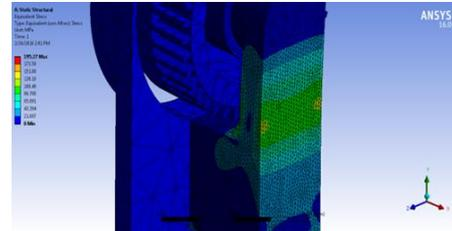
Figure.16. Von Mises in Bearing
