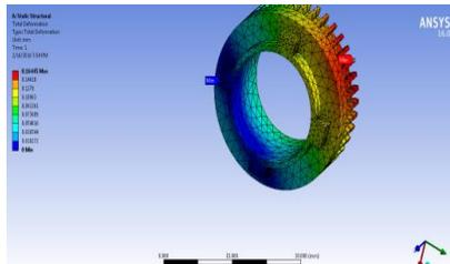
Figure.6. Deformation in Spline
