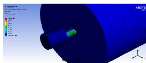
Figure.9. Von Misses Stress in Smaller Pulley
