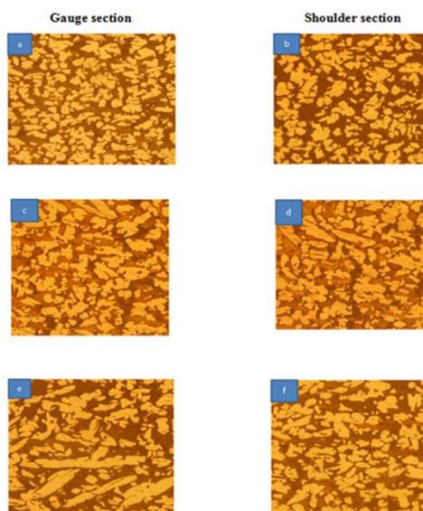
**Fig.3 (a), (c) and (e)** Optical micrograph of  $\alpha - \beta$  brass for gauge section and (b), (d) and (f) for shoulder section at  $500^\circ\text{C}$  and at strain rate  $1 \times 10^{-1} \text{ s}^{-1}$ ,  $1 \times 10^{-2} \text{ s}^{-1}$  and  $1 \times 10^{-3} \text{ s}^{-1}$
