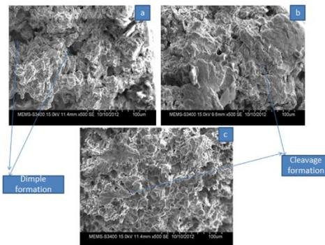
**Fig. 2 (a), (b) and (c).** Fractograph of  $\alpha - \beta$  brass at  $500^\circ\text{C}$  temperature and at strain rate  $1 \times 10^{-1} \text{ s}^{-1}$ ,  $1 \times 10^{-2} \text{ s}^{-1}$  and  $1 \times 10^{-3} \text{ s}^{-1}$
