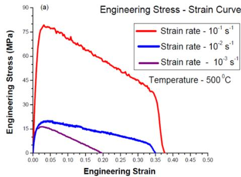
**Fig.1.** Engineering stress - engineering strain curve of  $\alpha - \beta$  brass at  $500^\circ\text{C}$  temperature and at strain rate  $1 \times 10^{-1} \text{ s}^{-1}$ ,  $1 \times 10^{-2} \text{ s}^{-1}$  and  $1 \times 10^{-3} \text{ s}^{-1}$
