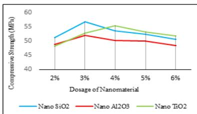
**Fig.2. 7 Days Compressive Strength of Nanomaterial Concrete**
