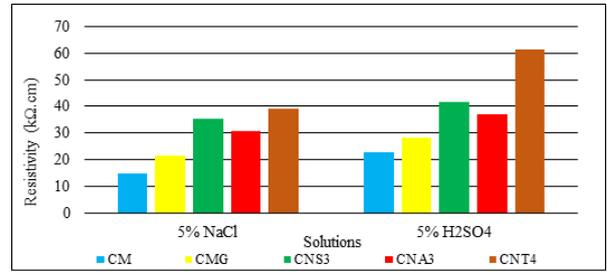
Fig.7. Graph for Electrical Resistivity in 5% NaCl and 5% H<sub>2</sub>SO<sub>4</sub> solutions
