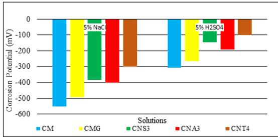
Fig.6. Graph for Corrosion Potential in 5% NaCl and 5% H<sub>2</sub>SO<sub>4</sub> solutions
