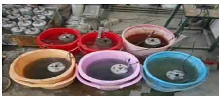
**Fig.1. Accelerated Corrosion of Cylinders**
