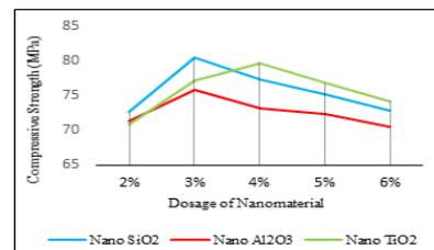
**Fig.3. 28 Days Compressive Strength of Nanomaterial Concrete**
