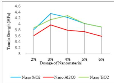
**Fig.4. 28 Days Tensile Strength of Nanomaterial Concrete**
