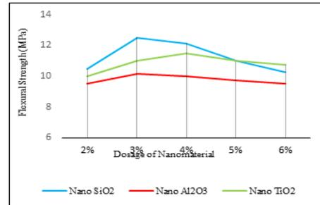
**Fig.5. 28 Days Flexural Strength of Nanomaterial Concrete**
