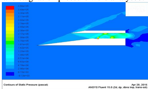
Figure.7. Pressure Contour for cowl angle 0 degree with micro cavity
