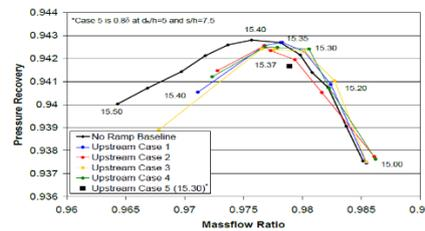
**Fig.3. Cane curves for upstream micro-ramp DOE study on A4 inlet geometry**
