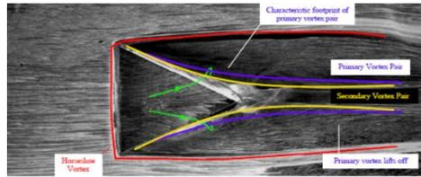
**Fig. 2 . Surface flow visualization of the features of the flow field around a single microramp. Freestream Mach number was 2.5 and the height of the ramp was 80% of the undisturbed boundary layer thickness.**
