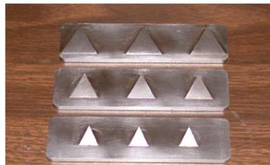
**Fig.4. Picture of three micro-ramp inserts from the experiment in the 15 x 15 cm supersonic wind tunnel**
