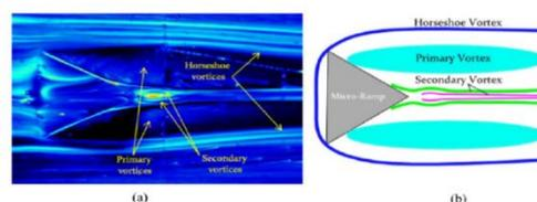
**Fig. 7. Surface flow visualization image and the vortex model given by Saad (2012)**
