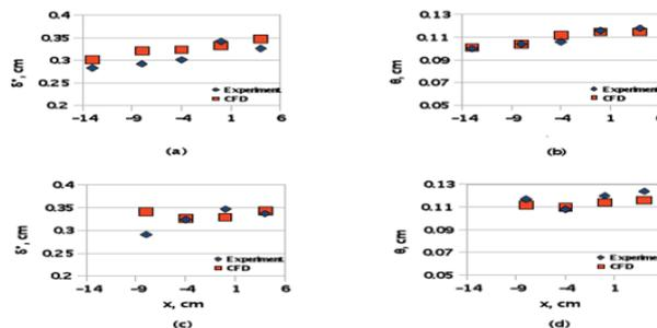
**Fig.5. (a) Empty tunnel compressible displacement thickness, (b) empty tunnel compressible momentum thickness, (c) micro-ramps only compressible displacement thickness and (d) micro-ramps only compressible momentum thickness along the stream wise direction.**
