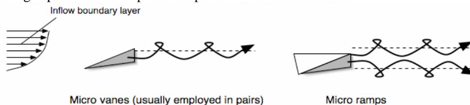
**Fig.1. Streamwise vortices generated by the micro-vortex generators (Lee sang, 2011)**
