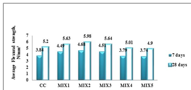
**Figure.3. Average Flexural Strength (7 and 28 Days)**
