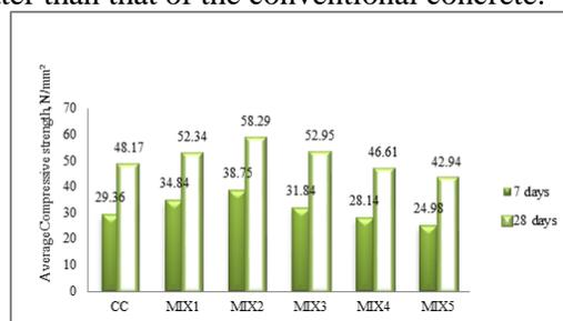
**Figure.1. Average Compressive Strength (7 and 28 Days)**
