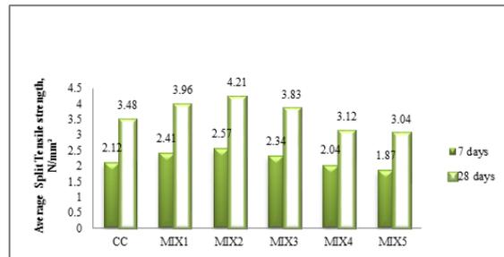
**Figure.2. Average Split tensile Strength (7 and 28 Days)**
