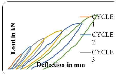
**Figure.4. Load – Deflection curve for for MIX2**
