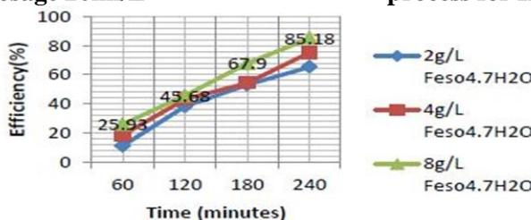
Figure.4. COD Removal Efficiency by fenton process for H<sub>2</sub>O<sub>2</sub> dosage 80ml/L
