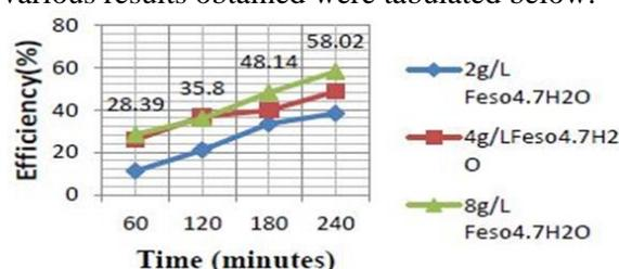
Figure.3. COD Removal Efficiency by fenton process for H<sub>2</sub>O<sub>2</sub> dosage 40ml/L
