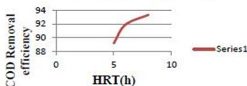
**Figure.6. COD Removal Efficiency BY integrated MBR**
