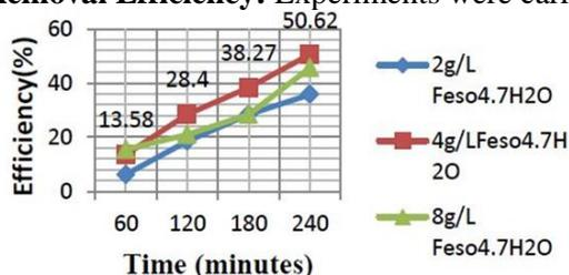
Figure.2. COD Removal Efficiency by fenton process for H<sub>2</sub>O<sub>2</sub> dosage 20ml/L
