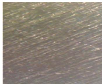
**Figure.5. Microphotograph of Al 6063 alloy with B<sub>4</sub>C 2%wt+red soil 6%wt**
