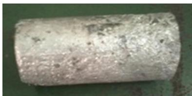
**Figure.2. Aluminum alloy6063+(B<sub>4</sub>C 4%wt+Red soil 6%wt)**
