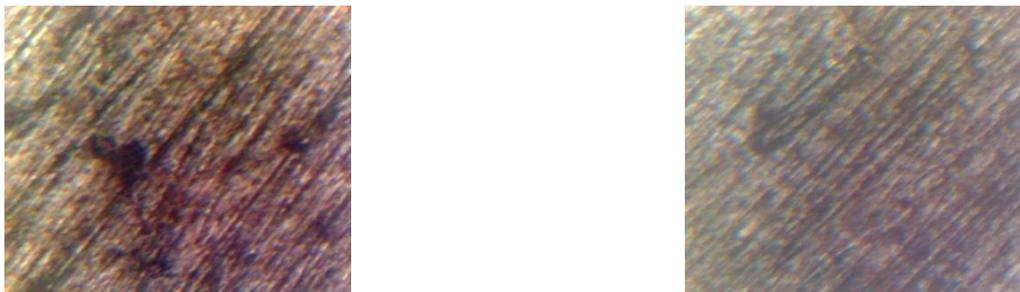
**Figure.6. Microphotograph of Al 6063 alloy with B<sub>4</sub>C 4%wt+red soil 6%wt**
