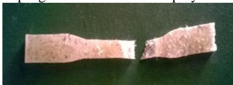
**Figure.6. Tensile test specimen after fracture**
