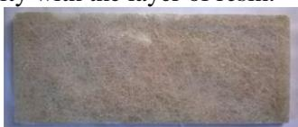
**Figure.4. Fabricated calotropis Glass fiber composite laminate**
