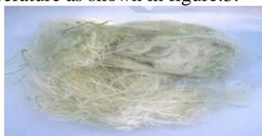
**Figure.3. Raw Calotropis fiber**
