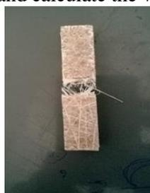
**Figure.7. Speciment after the impact test**
