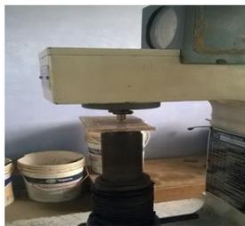
**Figure.5. Rockwell Hardness Machine**
