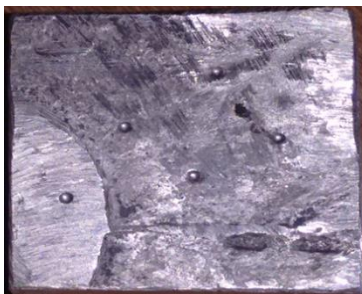
Figure.2. After Brinell hardness and Rockwell Hardness Test
