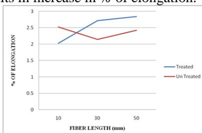
**Figure.3. % of elongation on fiber Length of the tensile strength with polyester resin**
