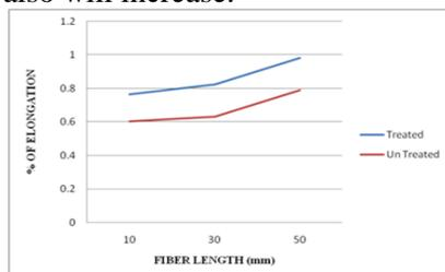
**Figure.1. % of elongation on fiber Length of the tensile strength With epoxy resin**
