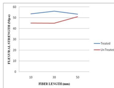
**Figure.6. Flexural strength on fiber length of the tensile strength with polyester resin**
