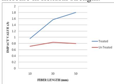
**Figure.7. Impact values on fiber length of the tensile strength with epoxy resin**
