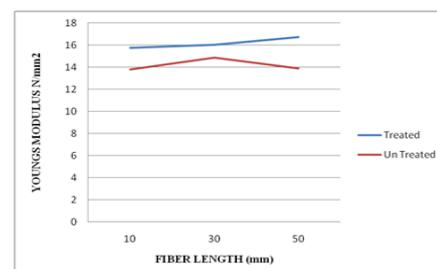
**Figure.4. Young's modulus on fiber length of the tensile strength with polyester resin**
