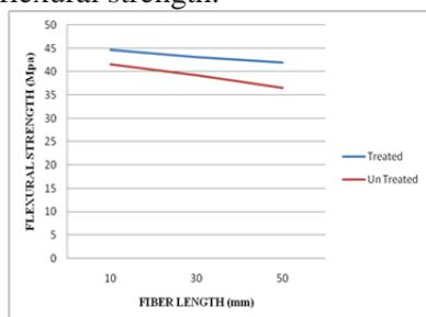
**Figure.5. Flexural strength on fiber length of the tensile strength with epoxy resin**
