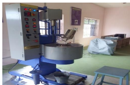
Fig.1. Stir casting setup
