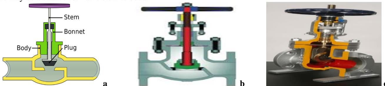
Fig.1. Parts of Globe valve (a, b, c)
