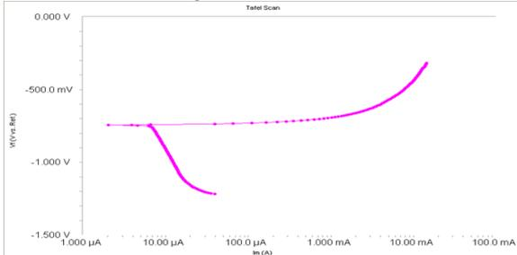
Figure.4. AA7175-T6 tafel polarization curve
