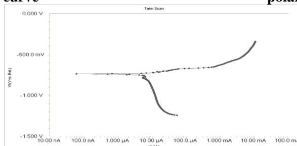
Figure.10. GTAW 160 Amps welding current tafel polarization curve
