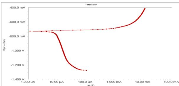
Figure.6. FSW 1000rpm welding speed tafel polarization curve
