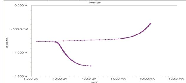
Figure.5. FSW 800rpm welding speed tafel polarization curve
