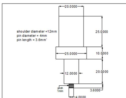
**Figure.2. Tool profile for FSW**
