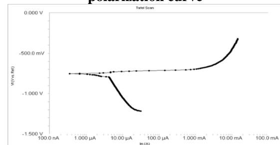
Figure.7. FSW 1200rpm welding speed tafel polarization curve
