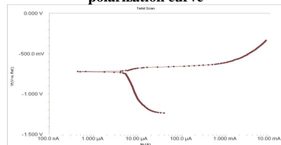
Figure.9. GTAW 120 Amps welding current tafel polarization curve
