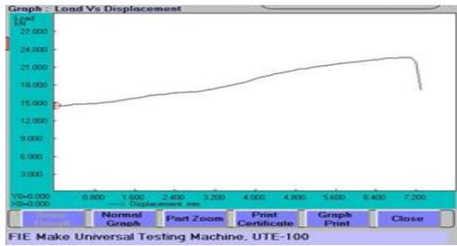
Figure.7. Graph for tensile test in base material of AA6061 (88%) with reinforcement of SiC (5%), Al<sub>2</sub>O<sub>3</sub> (5%), ZrO<sub>2</sub> (2%)
