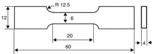
**Figure.5. ASTM Standard Size**
