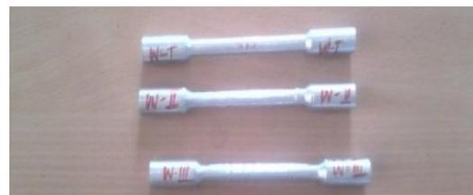
**Figure.6. Tensile test sample piece**
