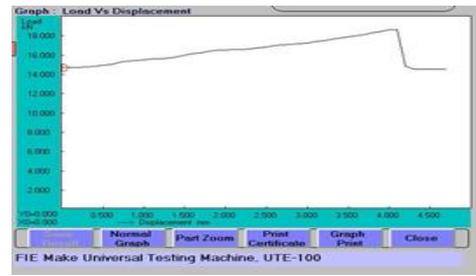
Figure.8. Graph for tensile test in base material of AA6061 (84%) with reinforcement of SiC (7%), Al<sub>2</sub>O<sub>3</sub> (6%), ZrO<sub>2</sub> (3%)
