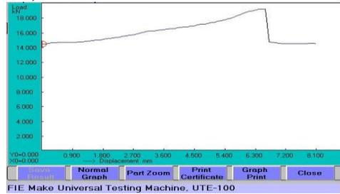
Figure.9. Graph for tensile test in base material of AA6061 (80%) with reinforcement of SiC (9%), Al<sub>2</sub>O<sub>3</sub> (7%), ZrO<sub>2</sub> (4%).
