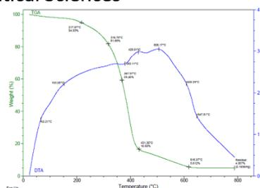
**Figure.1. TGA/DTA curve of rice husk and groundnut shell impregnated coir-polyester composites**
