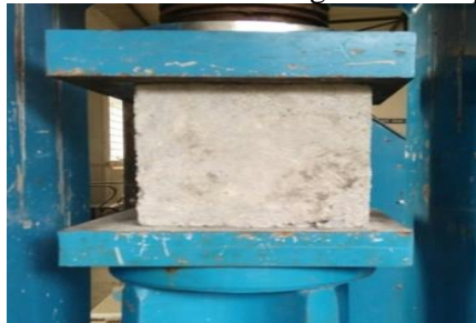
Figure.1. a) Compressive strength test
