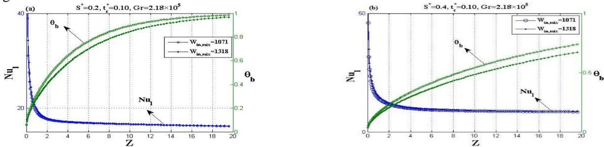
**Figure.2. Axial variation of local Nusselt number and Bulk fluid temperature**
