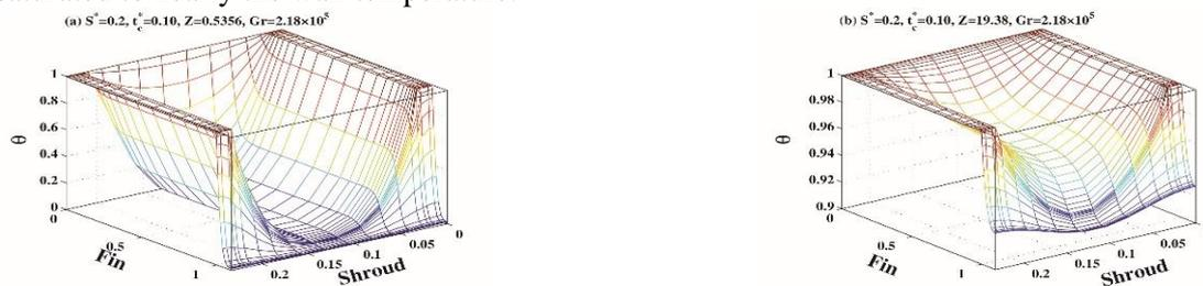
**Figure.3. Axial development of temperature profile**
