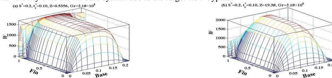
**Figure.4. Development of W- velocity profile**
