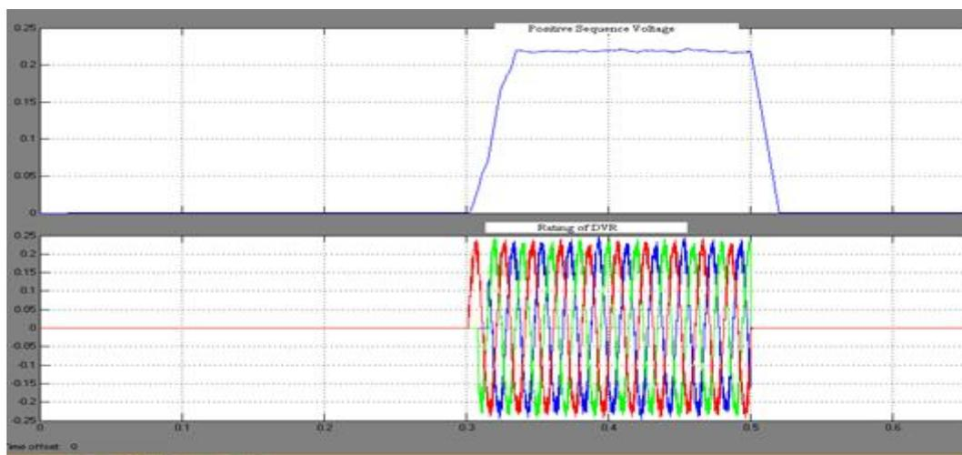
Fig.6. Simulation result of DVR voltage for compensation
