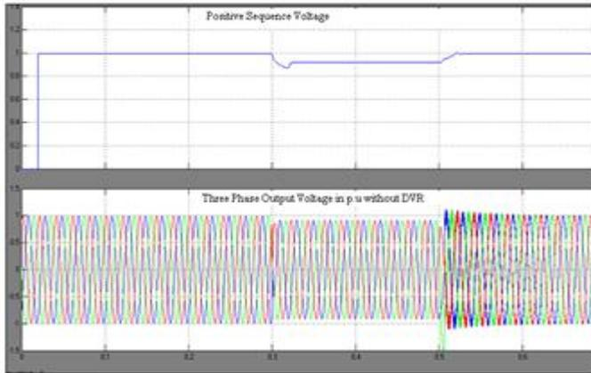
Fig.4 Simulation Result of output voltage without DVR
