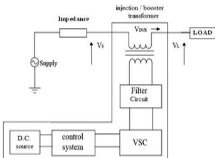
Figure 1. Schematic diagram of DVR
