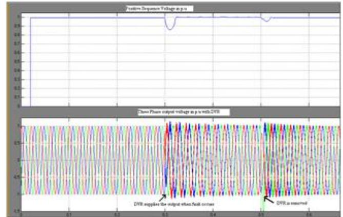
Fig.5 Simulation result of output voltage with DVR
