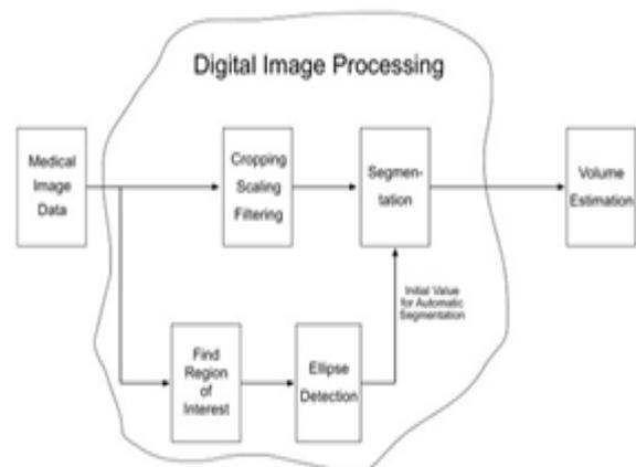
Figure.2.Block diagram of image segmentation
