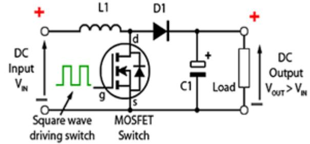
**Fig.6. Equivalent circuit diagram of boost converter**
