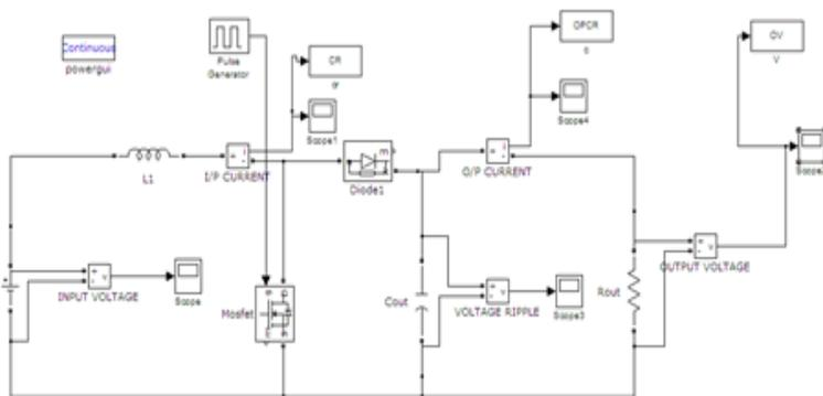
**Fig.7. Simulation of boost converter**
